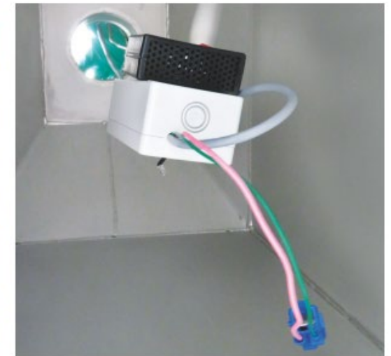
Open test chamber with integral ionisation head and moisture and temperature sensors.
