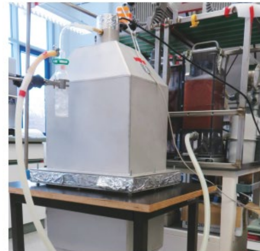
Earthed 60 L stainless steel test chamber with linked AGI-30 all-glass impinger.
